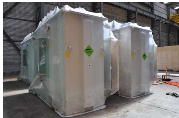
Figure 40: Nitrogen purged transformer furnished with gas cylinder
